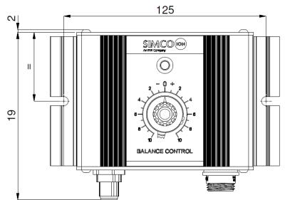
Fig. 2, Dimensions External Control Unit MPM
