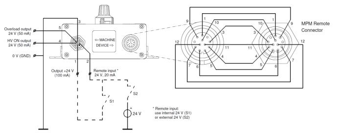
Fig. 3, External Control Unit - MPM connections.
