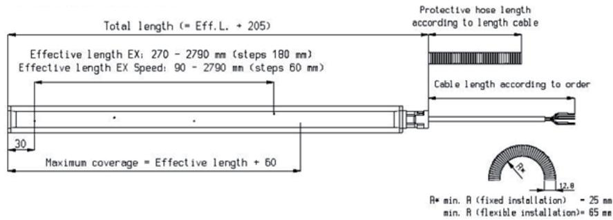
Technical drawing Performax Easy Ex (Speed) with PA protective hose
